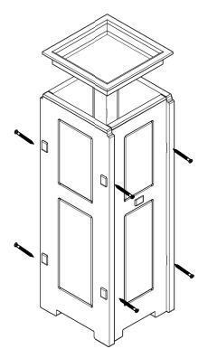
Insert screws into predrilled holes. Attach tray to top of ash urn.
