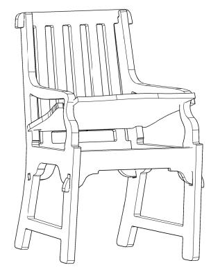
Insert front brace into holes in the legs. Keep the seat raised to allow the legs to spread so the brace will fit into holes. After the brace is in knock the seat down into place so it fits snug into place.
