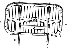
\*Attach 2-1/2" screws in 6 predrilled holes on edge of the top.
