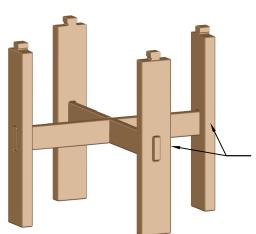
Assemble2 leg sections and insert into square holes in top
