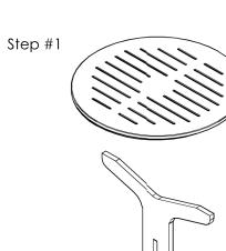
Attach the 2 legs together by sliding them into each other. The legs should be notched on opposite sides
